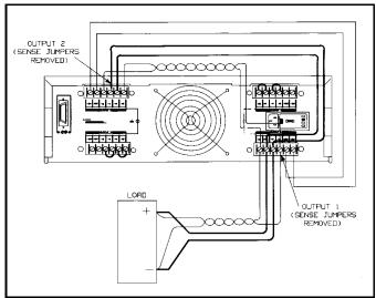
Figure 4-12. Parallel Connections with Remote Sensing
